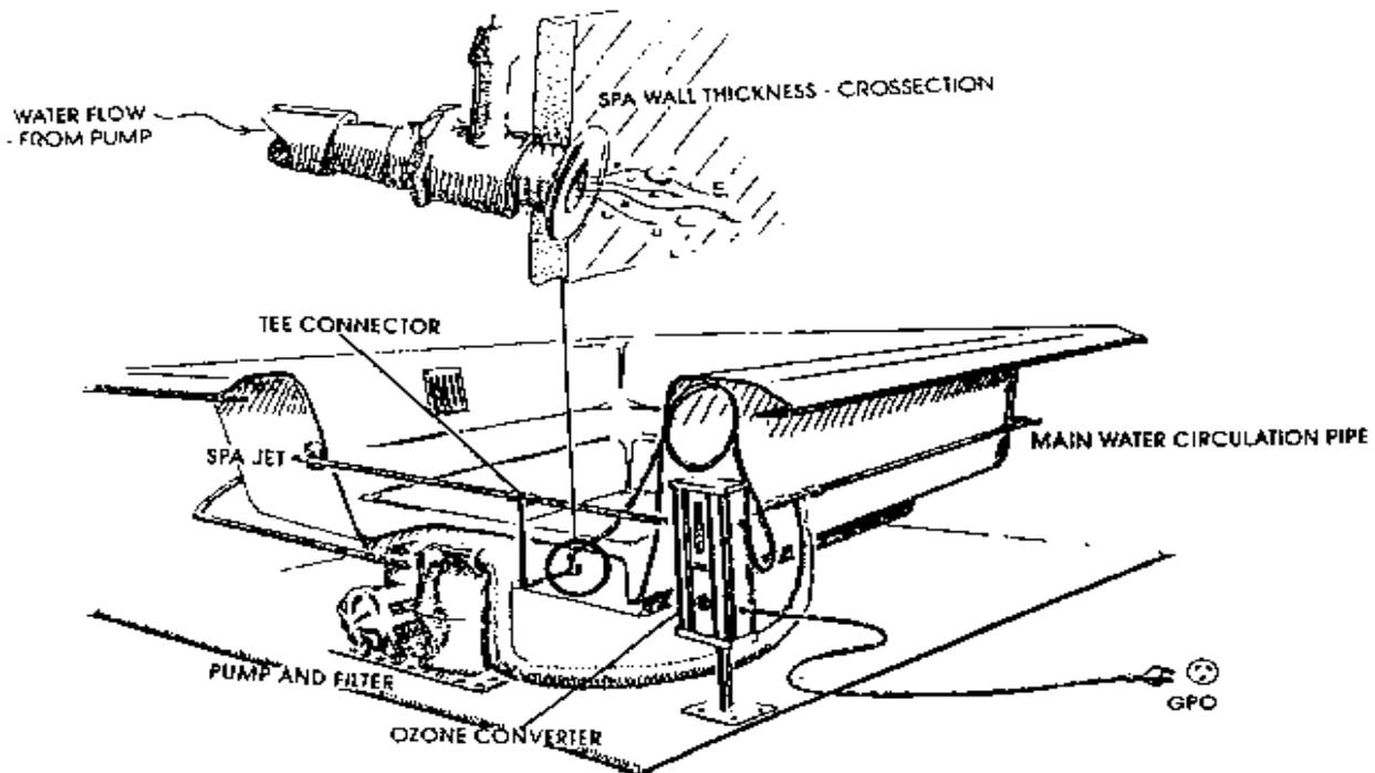
OZONE AIR LINE – MUST BE DOUBLE LOOPED AND CONNECTED ABOVE WATER LEVEL
