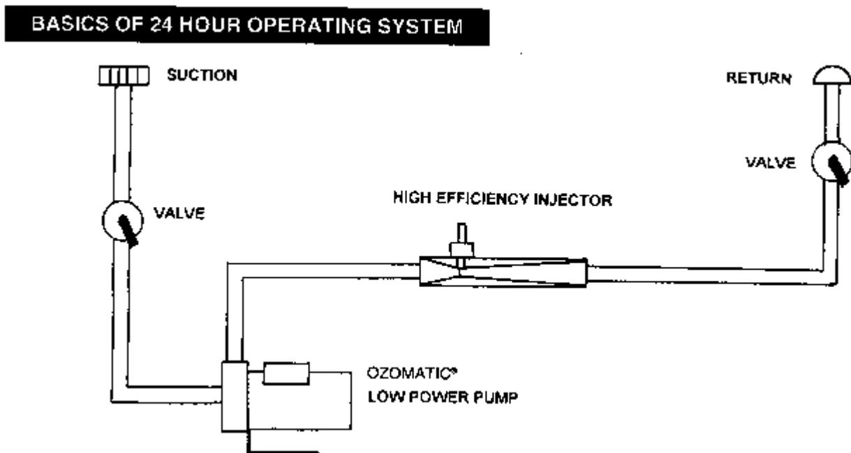
The Low Power Pump, High Efficiency Injector and Mini Footwell Injector all use 20mm (3/4") connections. Flexible 20mm (3/4") tubing should be used for all equipment - the Spa Suction/Return will need to be reduced down to this size.
