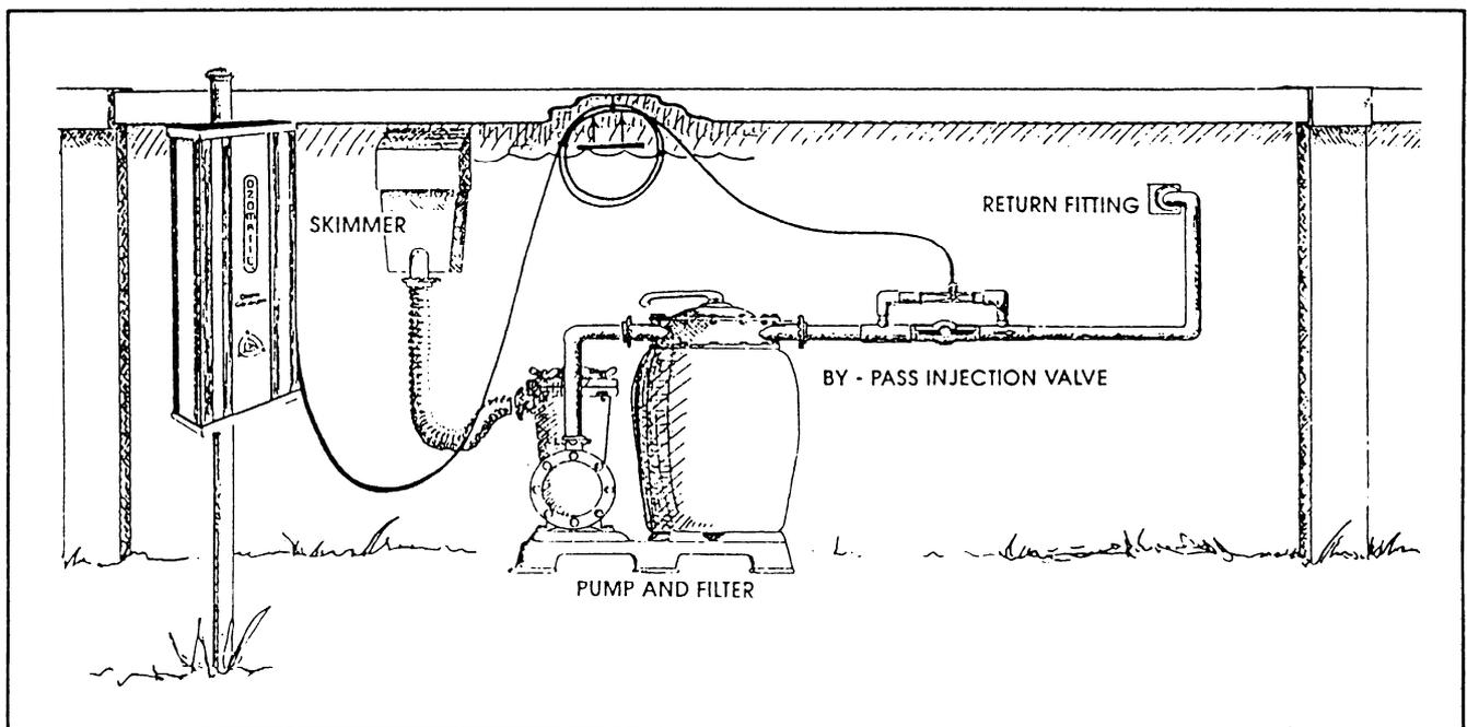
OZONE AIR LINE - MUST BE DOUBLE LOOPED AND CONNECTED ABOVE WATER LEVEL
